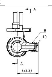
The ball valves did not leak during 82°C water temperature and 0.86 Kpa for 30 minutes.
