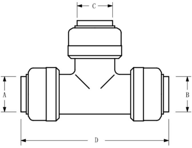
**Push-Fit Brass Tee** Maximum working pressure 200 psi
